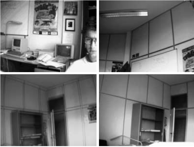
Fig. 4. Some of the images that were used for distortion calibration. Even blurred or fuzzy pictures can be used
