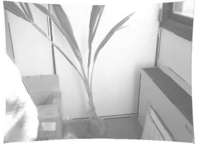
Fig. 5. A distorted image with the detected segments ( top ) and the same image at the end of the distortion calibration with segments extracted from undistorted edges ( bottom ): some outliers (wrong segments on the plant) were removed and longer segments are detected. This image represents the worst case, where some curves may be mistaken for lines
